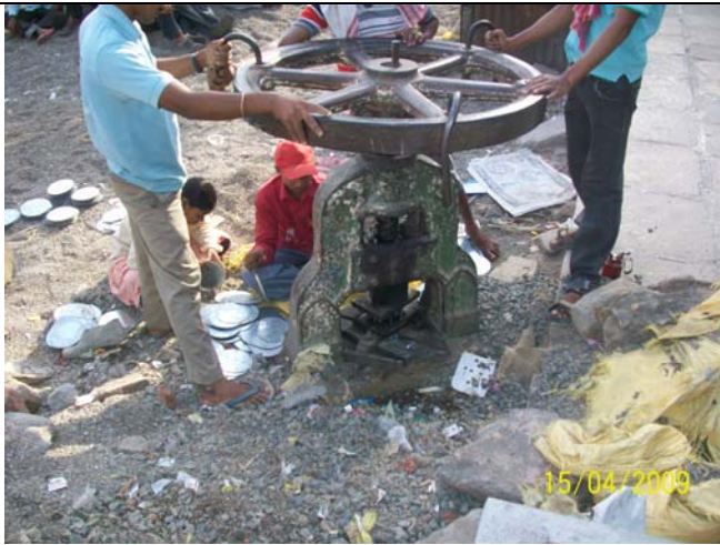
Students Preparing Dome joint plates
